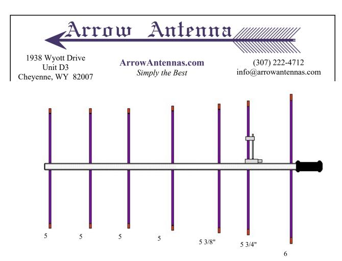
7 Element Portable Antenna for 70 cm
