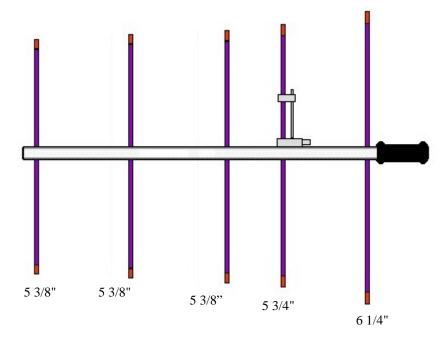
5 Element Portable Antenna for 70 cm
