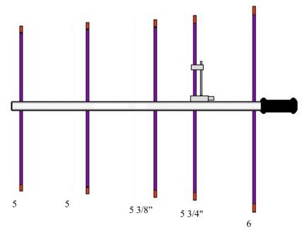
5 Element Portable Antenna for 70 cm
