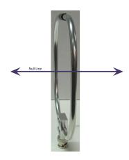
The Loop Antenna has the advantage of being less affected by reflection signals due to its Faraday shield.
